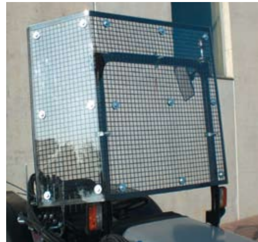
Protection net against worker's accidents
