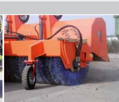
easy brush adjustment by adjusting-lever system
