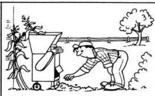
Don't clear discharge with hands. Never place any part of your body in discharge area.
