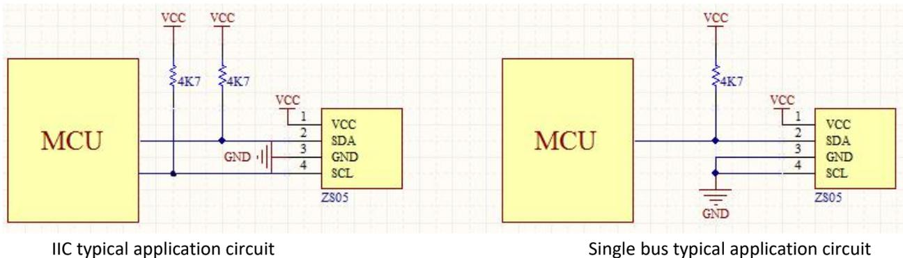
IIC typical application circuit
